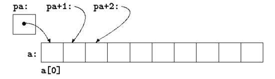
These remarks are true regardless of the type or size of the variables in the array a. The meaning of ``adding 1 to a pointer," and by extension, all pointer arithmetic, is that pa+1 points to the next object, and pa+1 points to the i-th object beyond pa.
