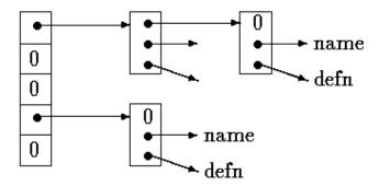
A block in the list is a structure containing pointers to the name, the replacement text, and the next block in the list. A null next-pointer marks the end of the list.
